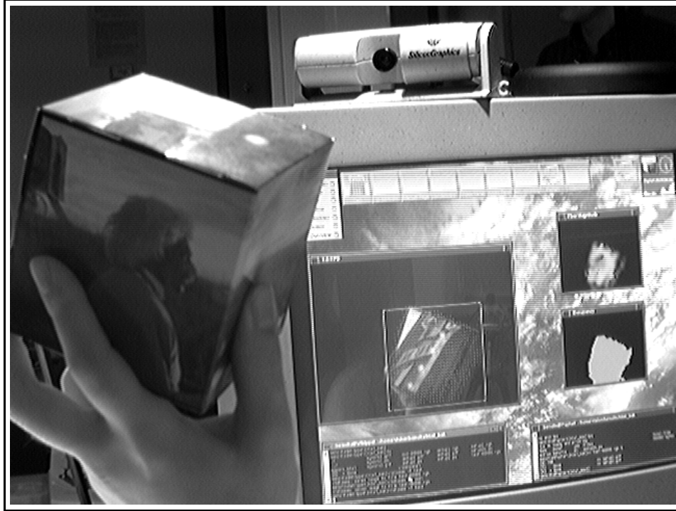
Figure 6: Laboratory set-up for building object models from optical flow measurements
