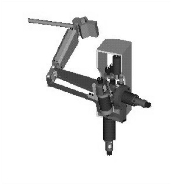
Figure 12: Freedom-7 Haptic Interface
