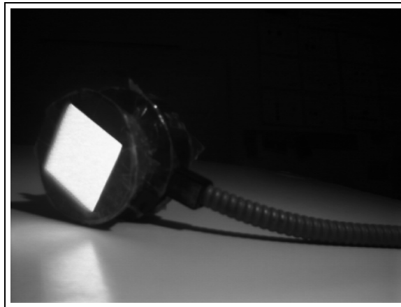
Figure 3: The prototype of the planar extended light source used in the active differential shape from shading experiment.
