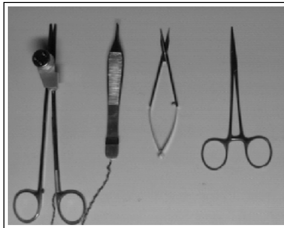
Figure 6.2: Instrumented surgical instruments used in the experiment
