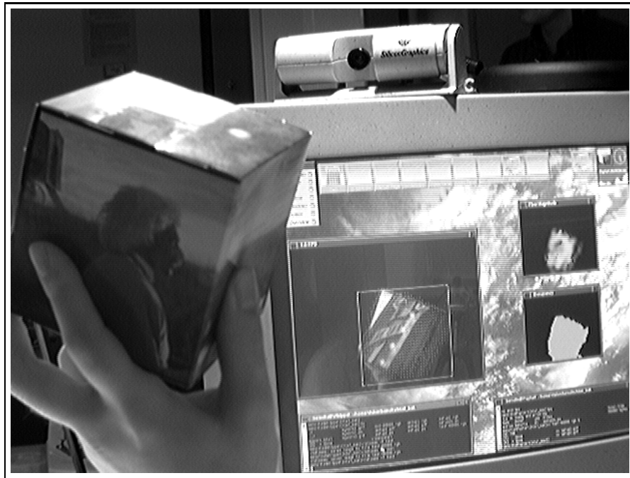
Figure 5.2: Laboratory set-up for building object models from optical flow measurements
