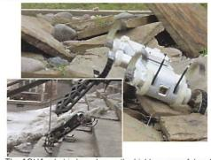
The AQUA robot is based upon the highly successful and mobile RHex platform. RHex is a small terrestrial walking robot that is capable of navigating rough terrain, climbing stairs, and running at speeds over 2.25m/s (5 mph). More information about RHex can be found at: www.rhex.net
