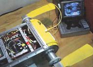
Images and data from AQUA's three onboard cameras and computer and transmitted along a single fiber-optic cable. This, along with AQUA's power autonomy allows for the use of a very small tether - greatly reducing drag.
