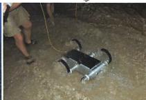
With terrestrial legs installed, AQUA can walk on land, and swim on the surface, allowing it to be launched from the surf zone.
