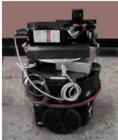
FIGURE 1.4. A picture of our mobile robot with the 2D laser range finder and the camera mounted on it.
